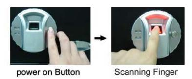
1. Press and release the **POWER ON BUTTON**, the red light (above the scanning window) will turn on. Put finger on the scanning window for recognition, remove finger when the red light turns off. The buzzer sound "Di", the green light will turn on then off and the door will unlock simultaneously.
